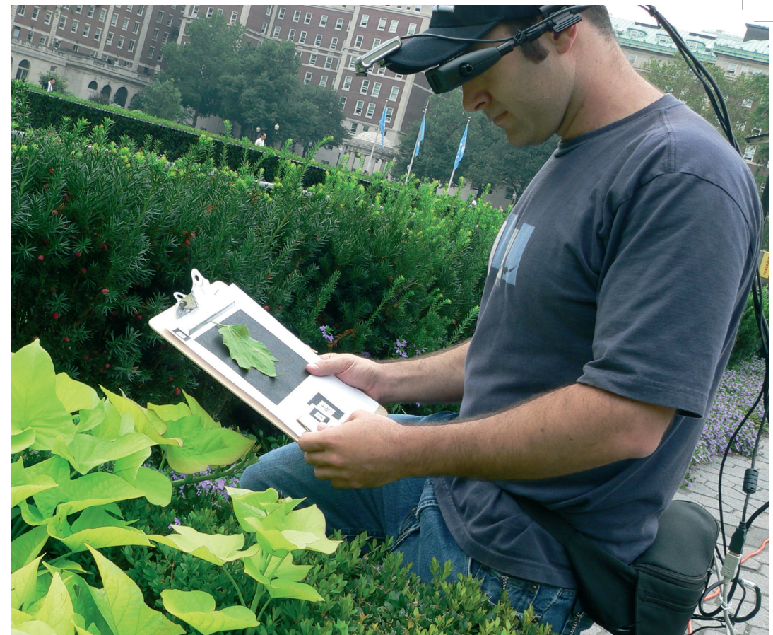
Augmented reality image of matching virtual leaves overlaid on physical scene as viewed through Sony LDI-D100B color, optical see-through, head-worn display. The image of the user's view was captured directly from inside the head-worn display, using a Toshiba remote lipstick camera and digitized at 720 x 480 resolution. Courtesy of Sean White.
