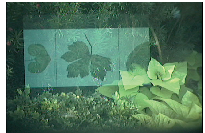
Augmented reality image of matching virtual leaves overlaid on physical scene as viewed through Sony LDI-D100B color, optical see-through, head-worn display. The image of the user's view was captured directly from inside the head-worn display, using a Toshiba remote lipstick camera and digitized at 720 x 480 resolution. Courtesy of Sean White.
